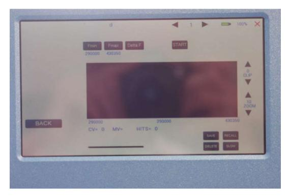
The values for Fmin, Fmax and Delta F will be set automatically according to the selected group. A touch on any of these buttons will have no effect. All other buttons can be used as described in the DIRP chapter.
