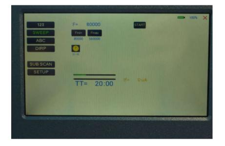
SWEEP can be used to swing for a limited time (standard 20 minutes) through a broad band of frequencies betw een a low er limit "Fmin" and an upper limit "Fmax". The step size "DELTA F" from value to value is defined automatically. "Fmin" and "Fmax" can be set by touching the icons Fmin and Fmax.
