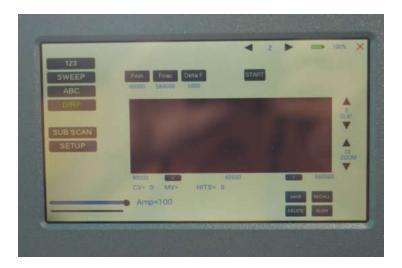
"DIRP" registers resonances to frequencies applied in steps of "DELTA F" within the limits between a lower value "Fmin" and an upper value "Fmax".
