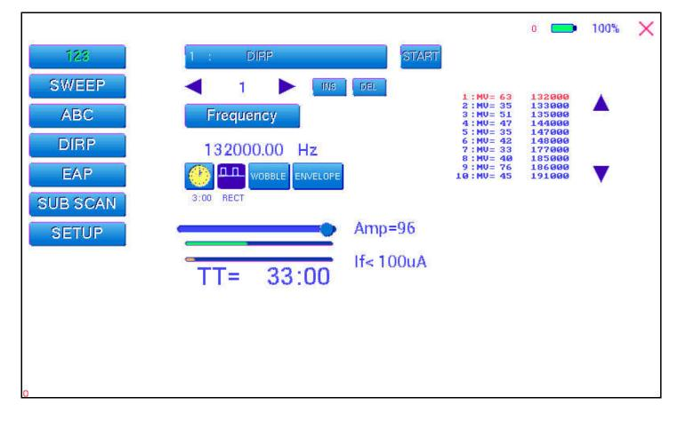
The menu "123" must be used to create and run individual programs with the ability to enter random frequencies in the range from 0.01 Hertz up to 15 MHz (Megahertz).
