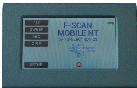
The F-SCAN MOBILE offers mobility and comfort. All settings and commands are entered with the display pen on the colored touch screen. The device has a multi signal output port for sine wave, adjustable square waves (full wave and dc-offset), smart wave. All connectors supporting applications are accessible from the front.
