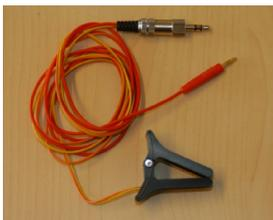
Interconnection cable for F-SCAN MOBILE, finger sensor Clip for DIRP.
